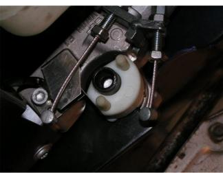
Assuming it is moving, remove the circlip you can see. Then undo the cable adjuster nuts right off to give you max slack. Remove the cables from the mechanism. Mark the face of the metal quadrant and with a bit of a wiggle (and perhaps some gentle levering with a screwdriver) the quadrant will slide off.
