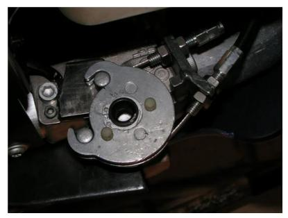
part with the cables attached. Just to check that it is the weak link broken and not a cable, move the raise lower lever to and fro and you should see this assembly moving. If it does, good – it is just the weak link broken. If not then, well its grief apparently.
